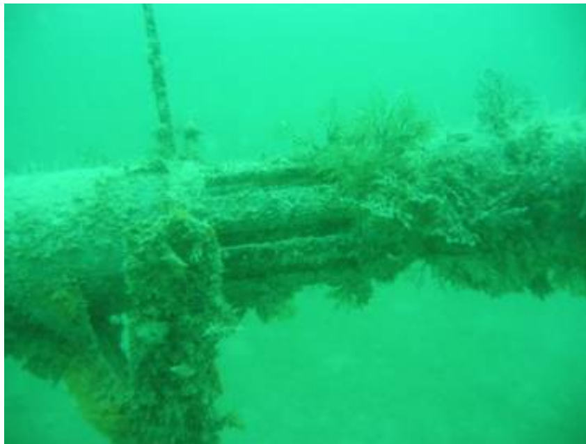
Figure 8: Typical bio-fouling on DO sensor after deployment for a couple of months.
