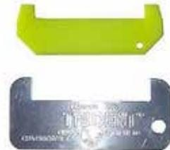
Lobster gauges must be in diver's possession and are used to measure the carapace, between the eyes to where the carapace meets the beginning of the tail. If the gauge is able to slide over carapace and move at all, the lobster is too small.
